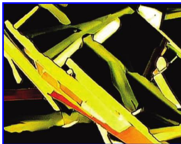
Figure 5.1. Characteristic optical microscopy texture, between crossed polars, of a smectic B liquid crystalline phase, showing typical bâtonnet texture: F10H10 at 57.5 °C, i.e., for the high temperature mesophase. From ref 259 with permission.
